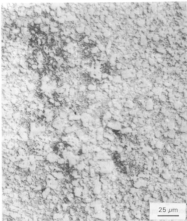
Figure 7 Optical micrographs of the Al-40Si composite (Sumitomo).
